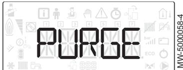
6. The venting cycle is run automatically on start-up of the appliance, if an error occurs or during **RESET** manual reset.
