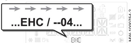
Central unit PCB **EHC-04**: direct circuit and domestic hot water
